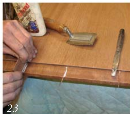
Photo 21 - 23, above, cracks in the lid edge are a common problem.
