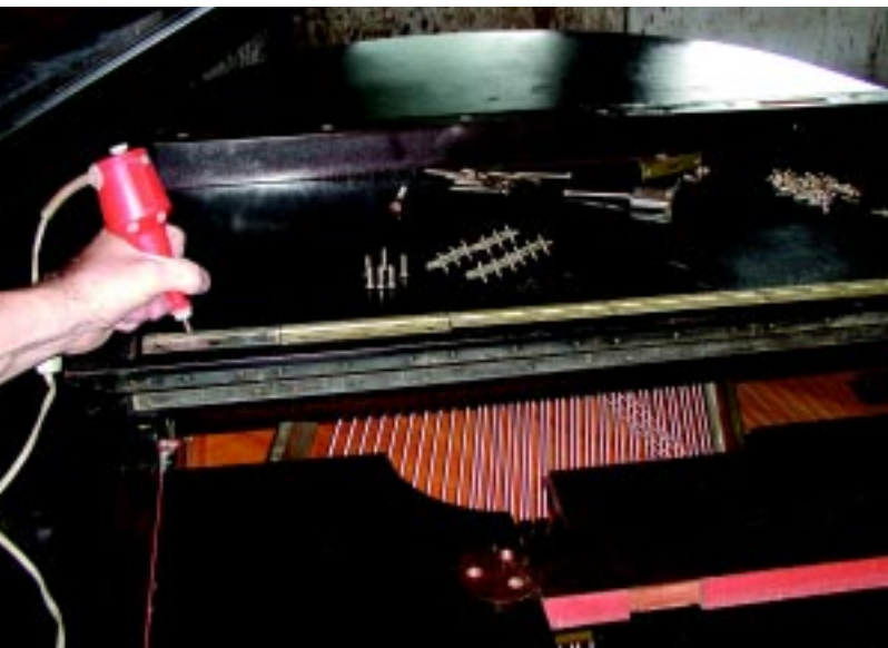
Photo 3 — The continuous lid hinge can be engraved on the back side to ensure proper reassembly.
