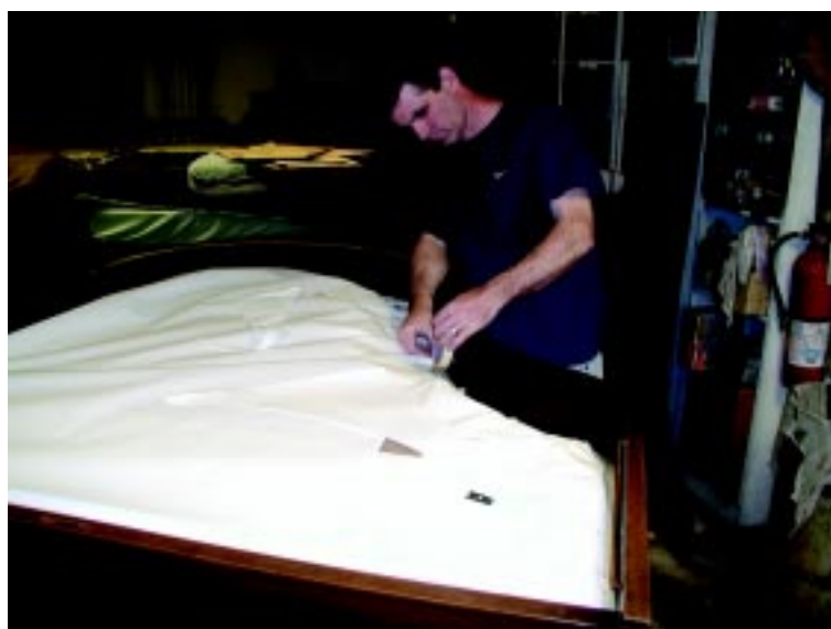
Photo 6 — A final layer of paper and tape protects the interior from harmful chemicals.
