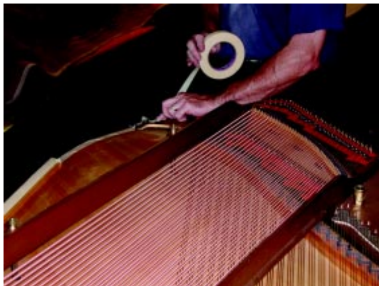
Photo 4 — Begin masking the interior by running a strip of masking tape around the perimeter of the soundboard.
