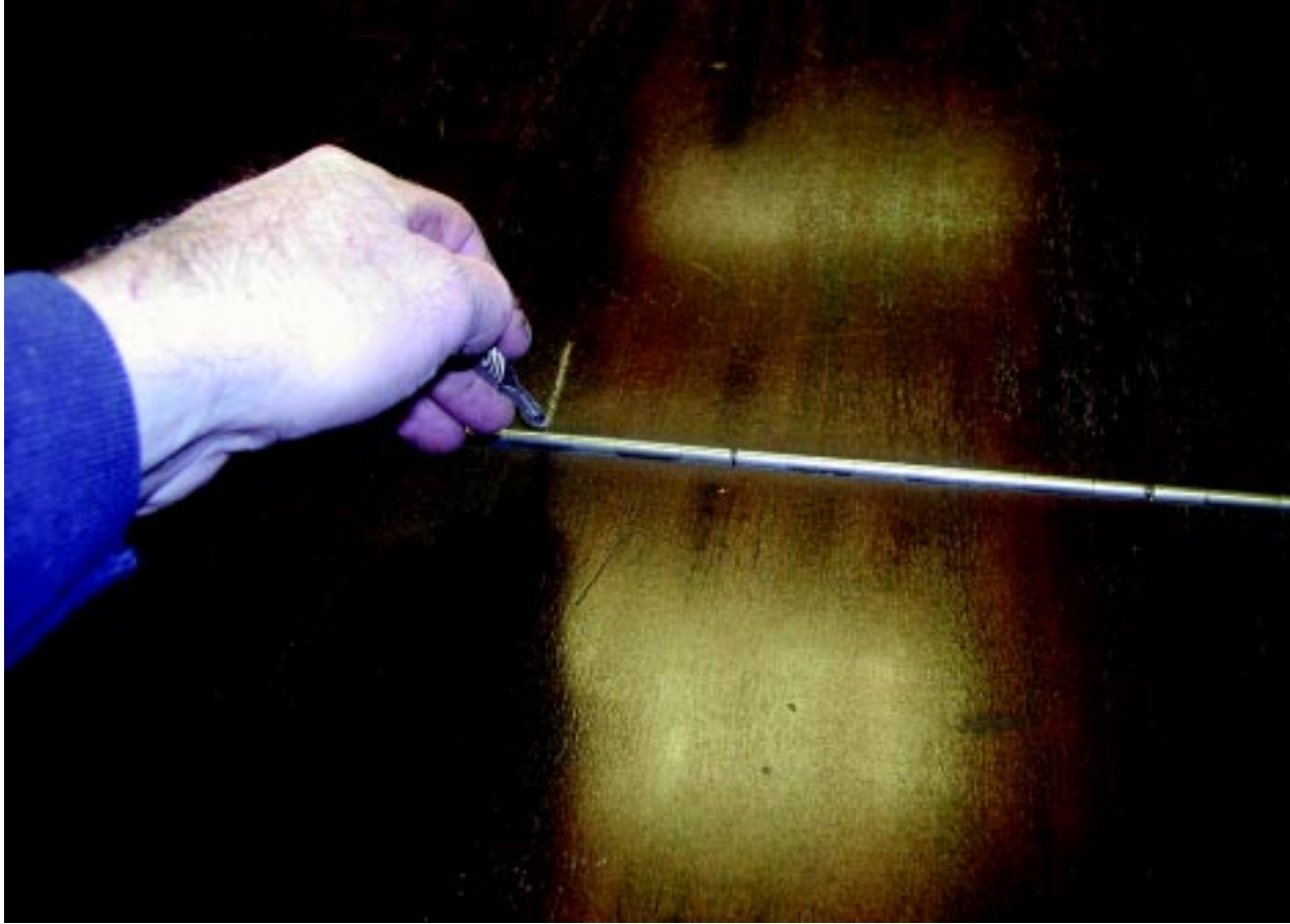
Photo 2 — Scored with a knife or saw, small cracks in the lid will be visible once finish is removed.
