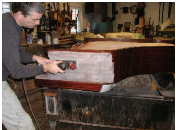
Photos 1 (TOP) and 2 (ABOVE) — Use a National Detroit 1100 in-line sander with 500-grit paper to cut the surface and remove any dust and finish shrinkage.
