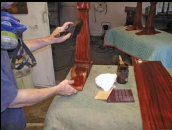
Photo 14 (top left) — Applying the glaze. Photos 15 (top right) & 16 (above left) — Spread glaze with brush or cheesecloth. Photo 17 (above right) — Remove excess glaze.
