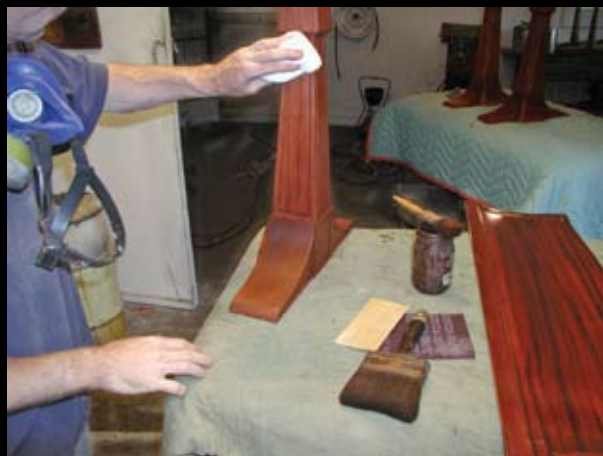
Photo 14 (top left) — Applying the glaze. Photos 15 (top right) & 16 (above left) — Spread glaze with brush or cheesecloth. Photo 17 (above right) — Remove excess glaze.
