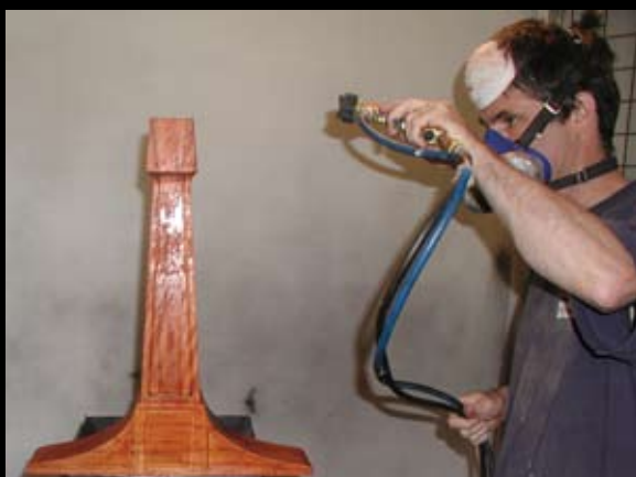
Photo 12 — Apply sealer coat.
