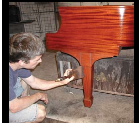
Photos 18 (TOP) & 19 (ABOVE) — Mounting the leg on the piano allows you to check color matching more closely.
