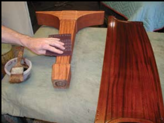
Photo 10 — Wipe with maroon Scotch-Brite to lighten colors as needed.
